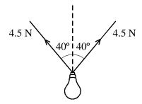
Calculate the magnitude of the resultant force exerted on the lamp by the wires.
